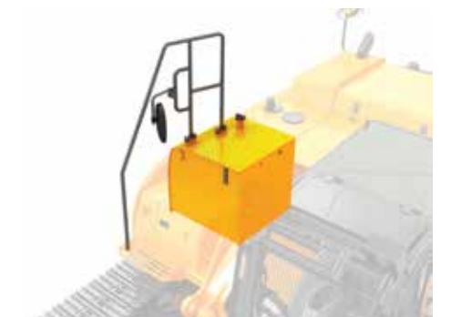
Handrail improvement (Side to top mounting)
