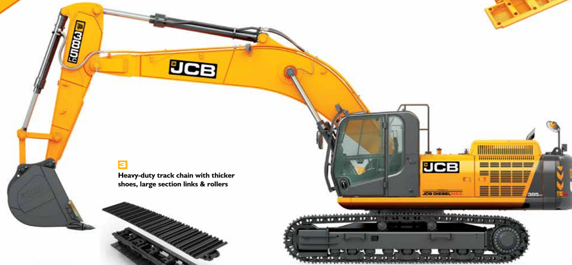
11 Heavy-duty special profile bucket for handling marble & granite blocks Quick fill quick discharge buckets 38T: 1.6, 1.8, 2.1 and 2.3 cu.m
