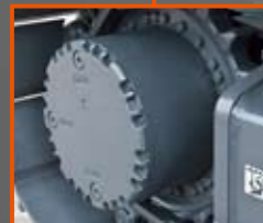
Stronger casing for travel motor
