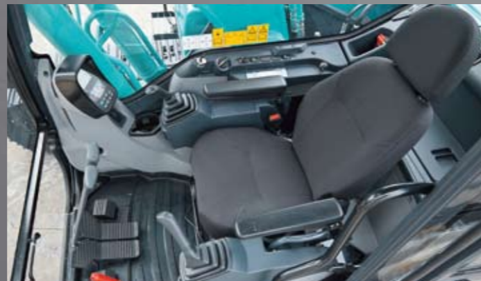
Seat can be reclined to horizontal position
